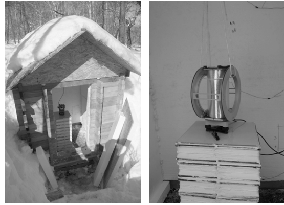
Figure 7. Vector/scalar Overhauser magnetometer POS-4. PET, Paratunka (Petropavlovsk).
