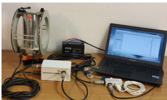
Figure 6. Vector/scalar Overhauser DNP magnetometer POS-4.
